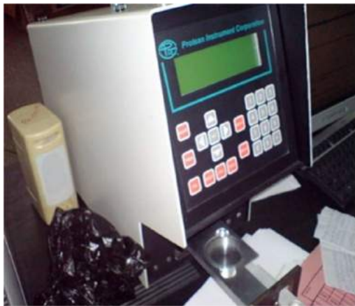
Fig. 3 MPC2000B-DP (machine for analysis gross alpha & beta).
